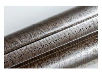
Figure 3.9. Close-up of the distinctive pattern on a Damascus-barrelled shotgun.
