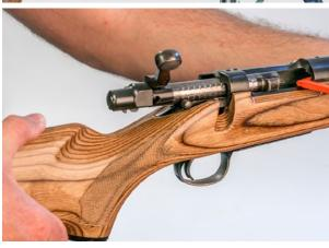
Figure 5.4. Top: cartridges removed from the magazine; Middle: physical check of the chamber; Bottom: chamber flag inserted.
