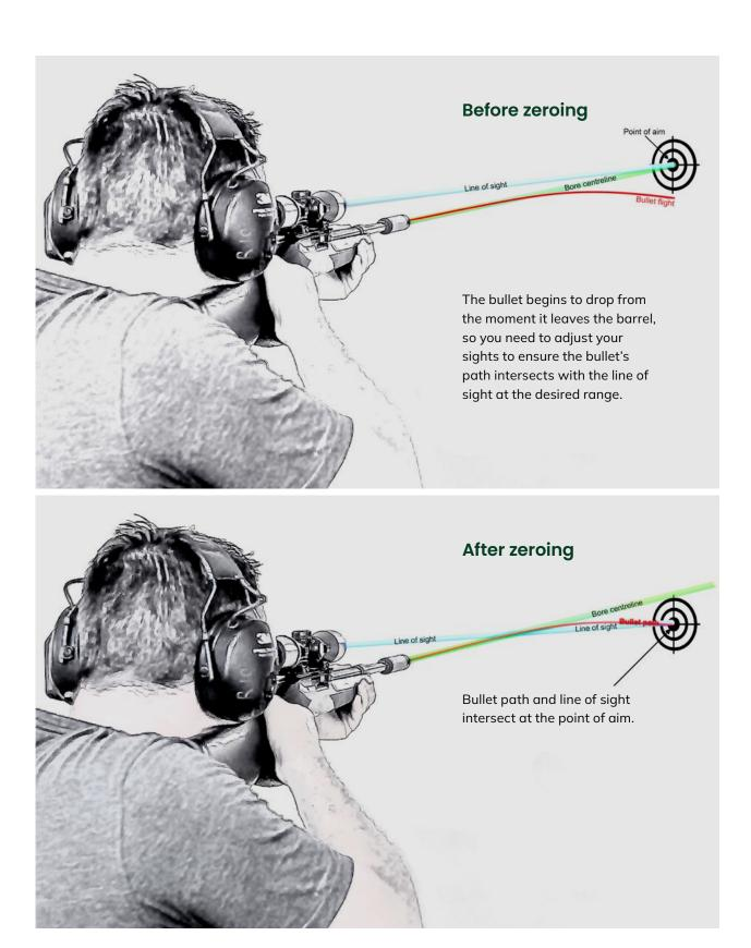
Figure 6.2. Zeroing – aligning the line of sight with the bullet path.
