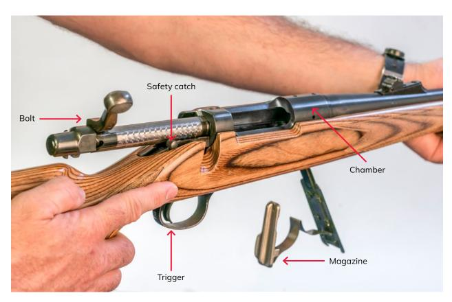
Figure 3.1. Close up of rifle action area showing common parts.
