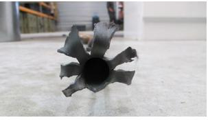
**Figure 7.4.** Images of a barrel damaged due to obstruction at the muzzle.
