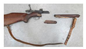
**Figure 4.19.** Damage caused by firing a cartridge into a barrel that was blocked by a squib load projectile that hadn't been removed from the barrel.
