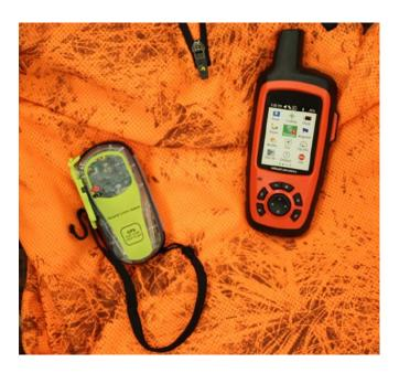
Figure 8.3. PLB on left, GPS on right.
