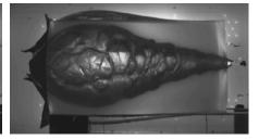
Figure 4.17. .308W 165gr Soft Point (SP) projectile. Left: Prior to penetration of the projectile; Middle: Initial expansion; Right: Final expansion.
