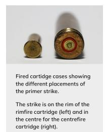
Figure 4.6. Rimfire and centrefire cartridges showing the different primer locations.
