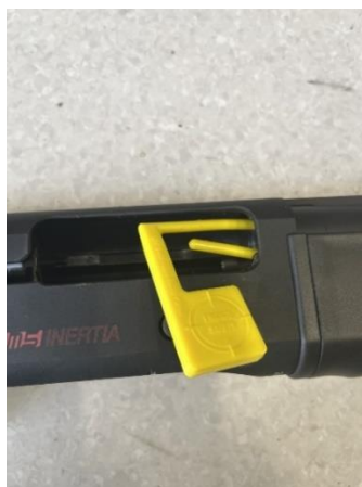
Example of a bent chamber flag rod being fitted into a shotgun chamber.
