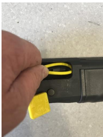
Example of a bent chamber flag rod being fitted into a shotgun chamber.
