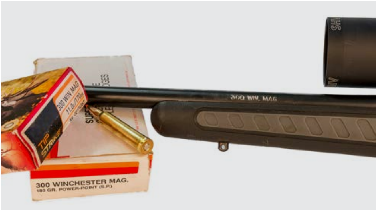
Figure 4.4. Cartridge identification information matching on the box, cartridge headstamp and barrel stamping.
