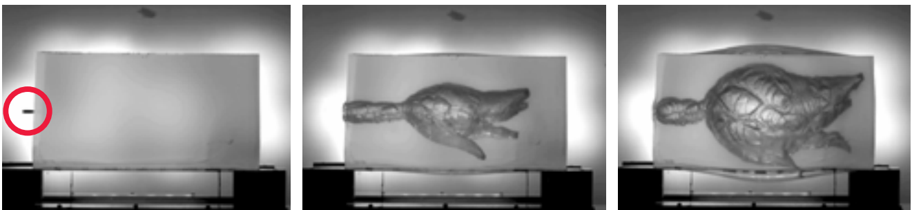
Figure 4.16. .308W 175gr Hollow Point (HP) projectile. Left: Prior to penetration of the projectile; Middle: Initial expansion; Right: Final expansion.
