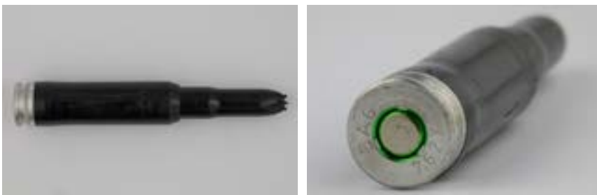
Figure 4.15. Blank rifle cartridge showing plastic case (left) and live primer (right).
