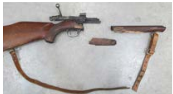
Figure 4.19. Damage caused by firing a cartridge into a barrel that was blocked by a squib load projectile that hadn't been removed from the barrel.
