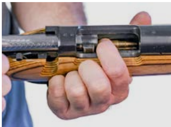
Figure 5.1. Firearm in the load state. Note cartridges are in the magazine, but the chamber is empty.
