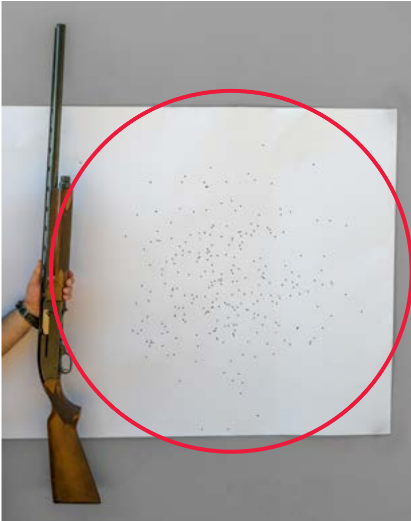
Figure 6.3. Shotgun pattern – modified choke at 20 metres.
