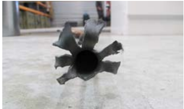
Figure 7.4. Images of a barrel damaged due to obstruction at the muzzle.
