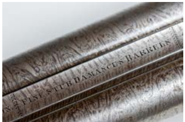
Figure 3.9. Close-up of the distinctive pattern on a Damascus-barrelled shotgun.
