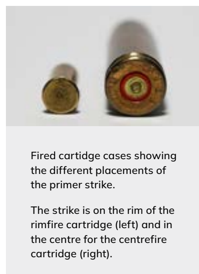
Figure 4.6. Rimfire and centrefire cartridges showing the different primer locations.
