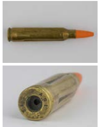
Figure 4.13. Drill round showing the orange polymer projectile, fluted case and no primer.
