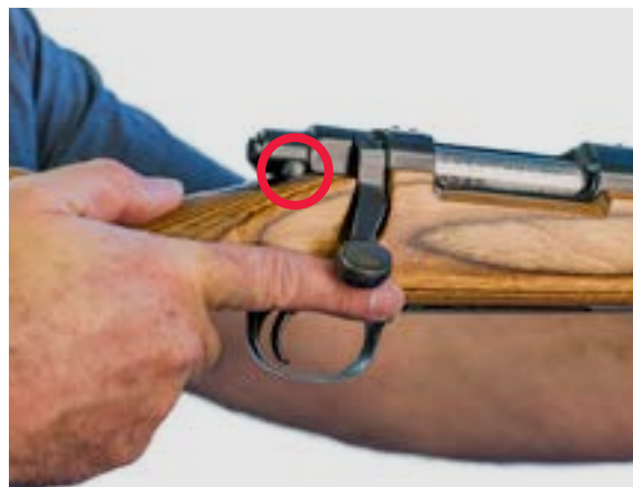
Figure 5.3. Bolt is closed on a chambered cartridge, safety catch is 'off' ('fire'), causing the firearm to be in the Instant state.
