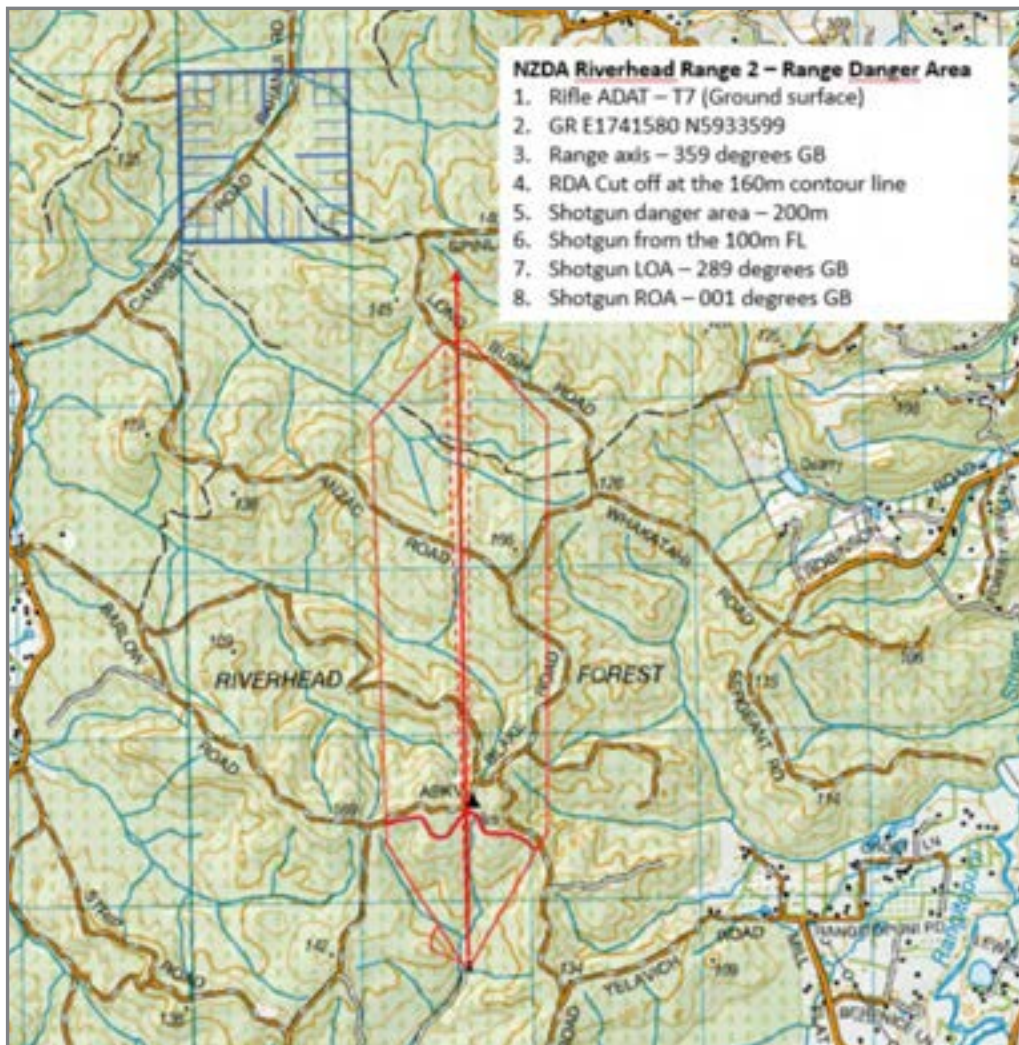
Figure 4.4 – Electronic application of an ADAT to produce a scale diagram of the range danger area with the reduced danger area indicated by the red bold line using the Microsoft PowerPoint software application
