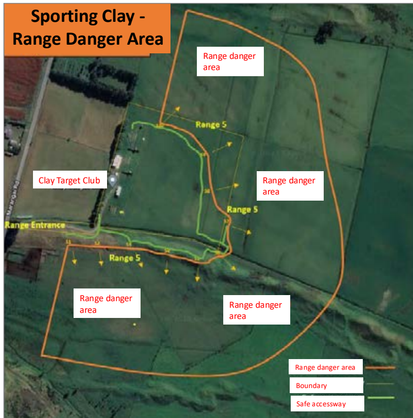
Figure 2.8 – Example of a sporting clay shooting range with an ammunition danger area template applied to establish the range danger area
