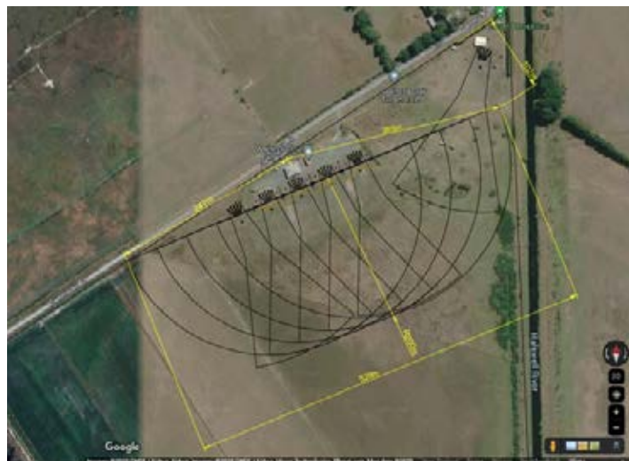
Figure 2.7 – Example of a combined skeet and down the line (DTL) trapshooting (field) range with an ammunition danger area template applied to establish the range danger area
